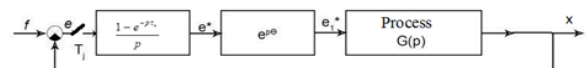
Figure 2. Equivalent circuit of a pulse-frequency system with a delay of the control signal
